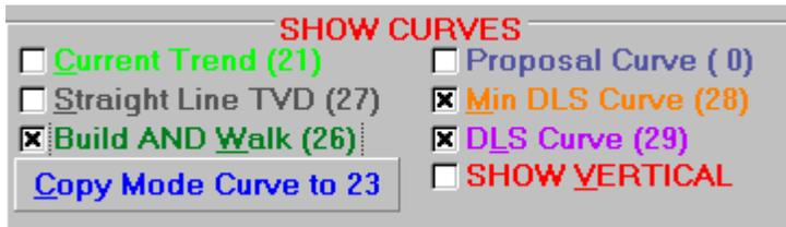
The SHOW CURVES area of the screen is reproduced to the left. By checking the boxes the user is able to display more than one projection at the same time. Note the Curve #'s in parentheses
