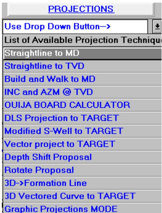
The list of available Projection techniques can be seen by clicking on the drop down button. These may be used to extend the well profile by sequential stages, and are generally the same as described in WinSERVE Projection Methods. The use of these methods is illustrated by means of examples later in this section. In addition, there are two tools found in this menu that are not projections, but can be useful on occasion for well plans with a 2-D Tie In:
