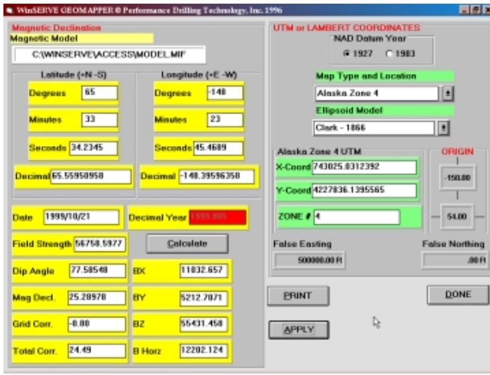
The Geomapper is designed to assist the user in calculating the UTM and Lambert coordinates from latitude and Longitude, or vice versa. Once the geographical coordinates are calculated the magnetic declination and grid correction are calculated and displayed. This program uses the same methods of calculation as the Department of Defense program GEOMAG. The calculation of the Map Projections are taken from the U.S. Geological Survey Professional Paper 1395.
