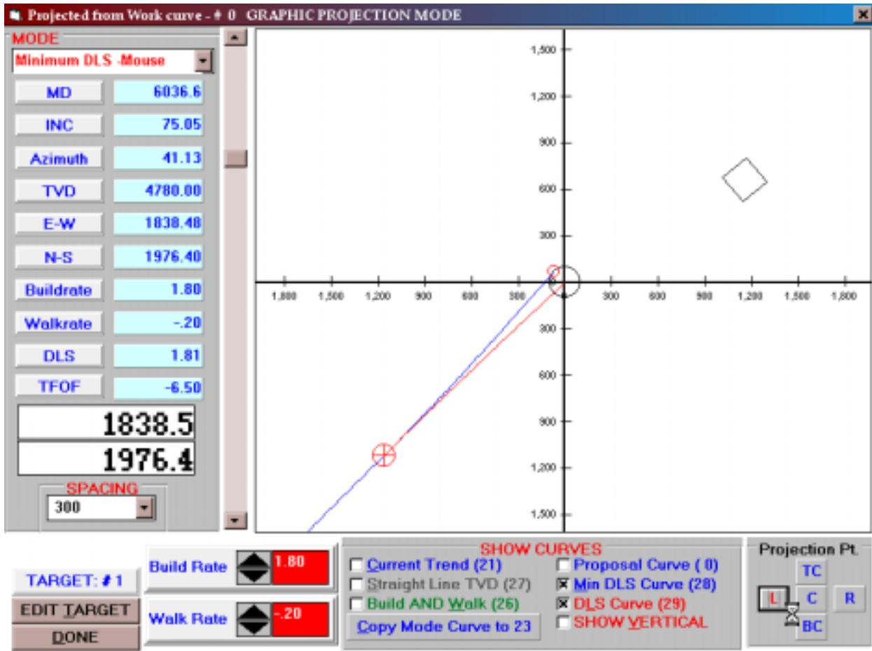
The Graphical Projection mode allows the user to do complex projections by simply pointing and clicking with the mouse. Shown above is an example of the screen accessed by pressing the PROJECT button (Binoculars icon) on the Main Screen. Projections are made from the workcurve as identified by the Work #, as the user is reminded by the banner at the top of the screen, either from the SENSOR or BHL Location as selected on the Main Screen.
